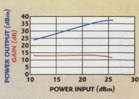
▲ Fig. 5 The device's power output and gain vs. power input.
